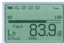
Adds frequency band switching analyzer function to sound level meter.
