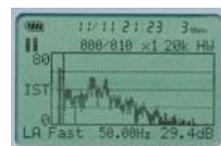
Adds FFT analyzer function to sound level meter.
