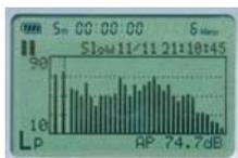
Adds 1/1, 1/3 octave real-time analyzer function to sound level meter.
